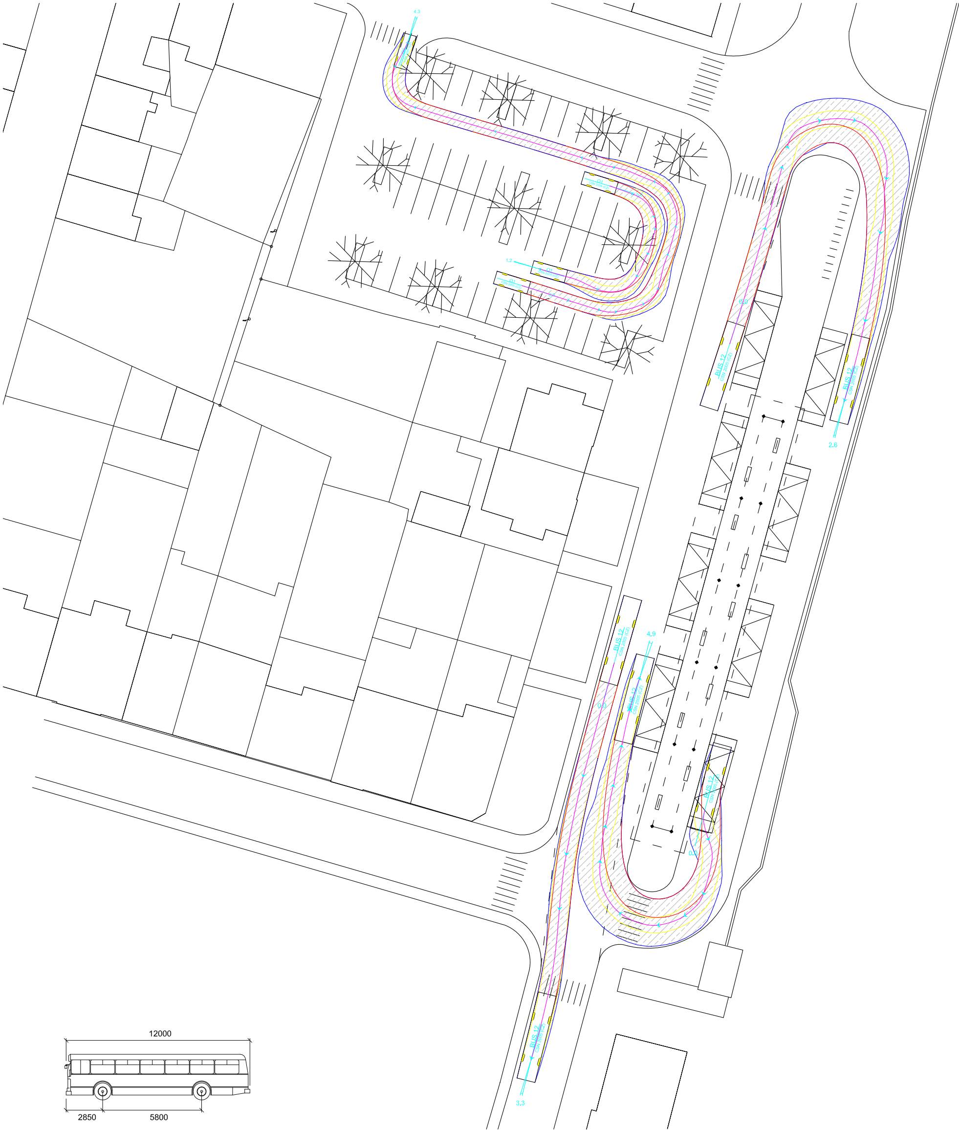
BUS 12 mm Width : 2500 Track : 2500 Lock to Lock Time : 6.0 Steering Angle : 50.9
